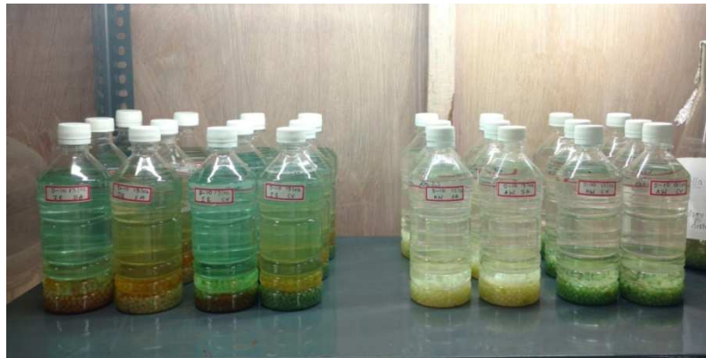
Figure 2: Bottles Containing Waste Water Samples Inoculated with Immobilised Scenedesmus Abundans and Chlorella Vulgaris Cultures
